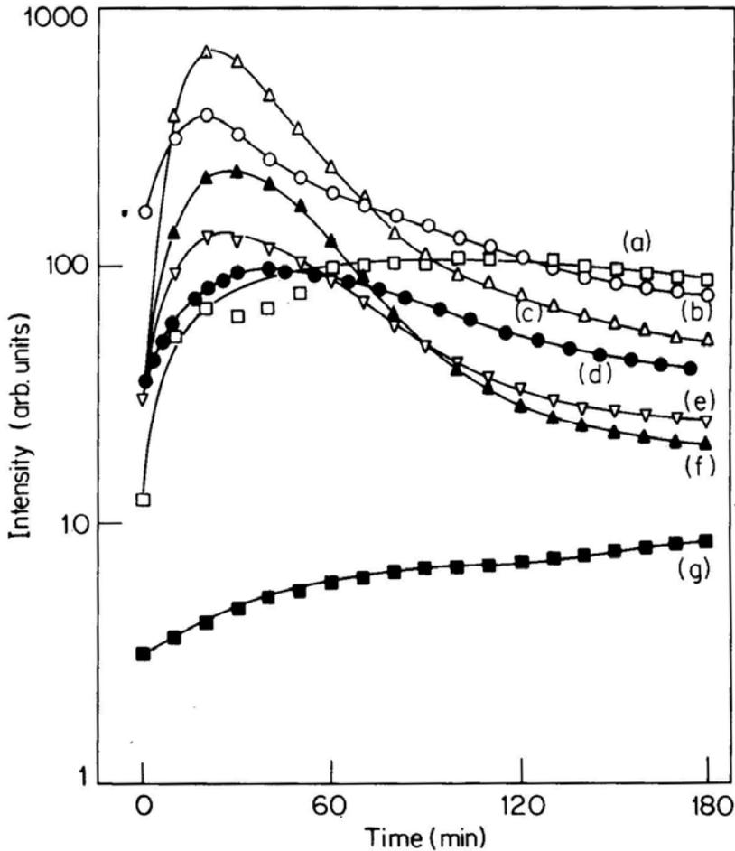
**Figure 7.** Plot of light intensity versus time for a sample which had been kept in water for different intervals of time before measurements.
