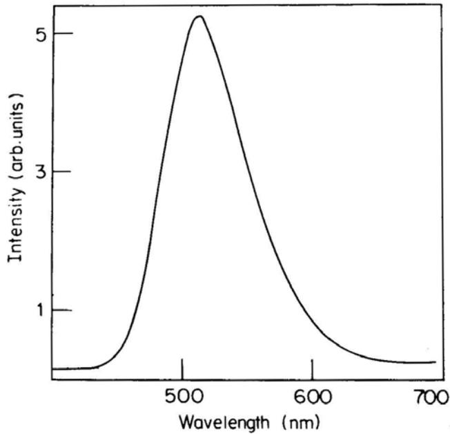
**Figure 3.** The emission spectrum of the luminous wood.
