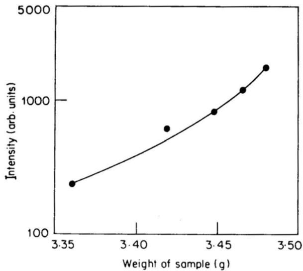
**Figure 2.** The dependence of light intensity on water content of the sample.
