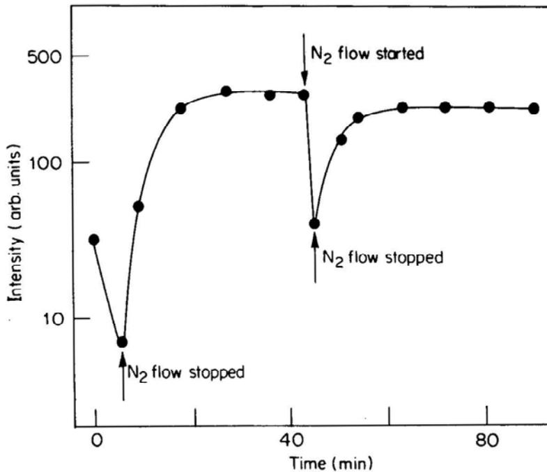
**Figure 4.** Effect of the presence of N<sub>2</sub> gas on the light intensity.
